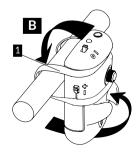
You can now connect the cell to the preAmp (« simple » mounting) or to the coupler and then connect the coupler to the preAmp input using the MCX extension cable (mounting « with coupler »).
