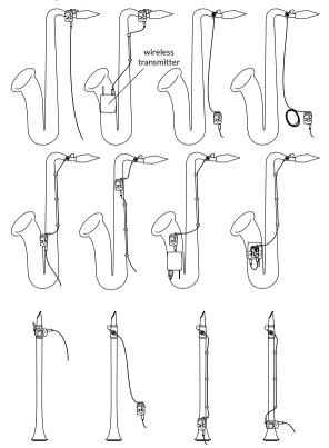
The preAmp can also be belt-worn, pocketed, left on the ground or attached to a wireless transmitter. Elastic hooks will let you attach a transmitter on your saxophone's bell for instance.
